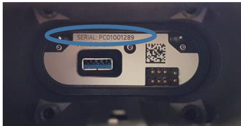
Serial and Pin numbers located in the 'tail' of the OZO
