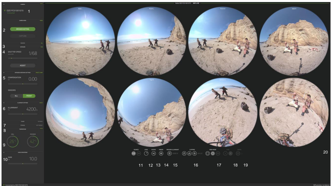
OZO Remote V1.4.0 UI showing images from the 8 cameras
